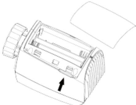
The service life of new alkaline batteries is approximately 1.5 years. A battery symbol (bat) on the display indicates that the batteries need to be replaced. After removing the empty batteries, wait approx. 1 minute before inserting the new ones. This device does not support operation with rechargeable batteries.
